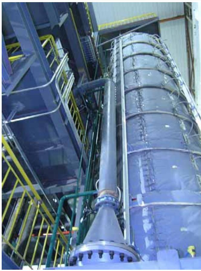
Neutron Counter at the Sudbury Neutrino Observatory – NASA employed CVMR® to Build a Pure Nickel Exoskeleton for the Vessel
